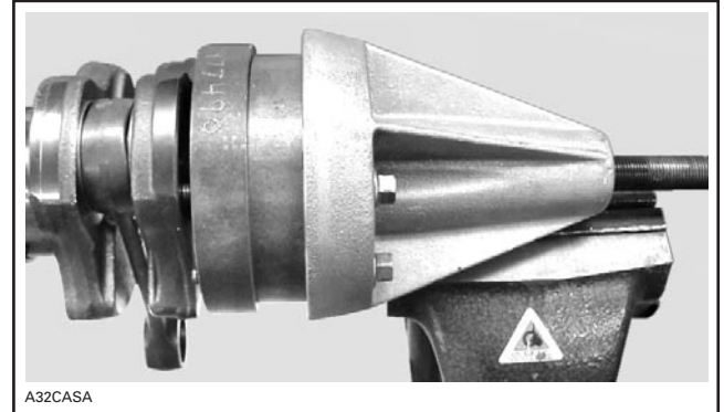
BEARING PULLER SECURED IN THE VISE
