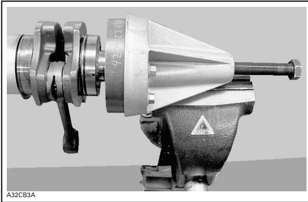
BEARING PULLER SECURED IN THE VISE
