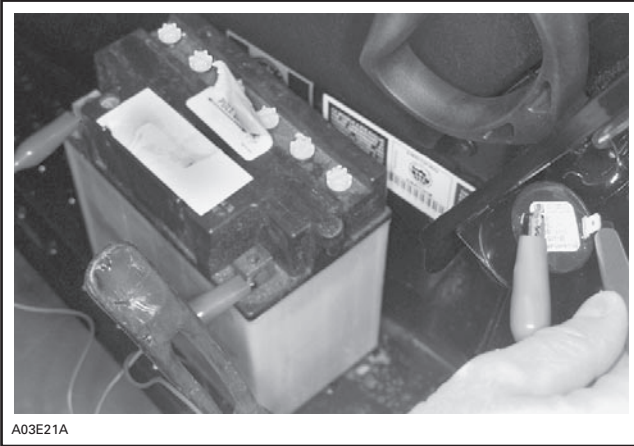
12-VOLT BATTERY PLUGGED TO BUZZER
