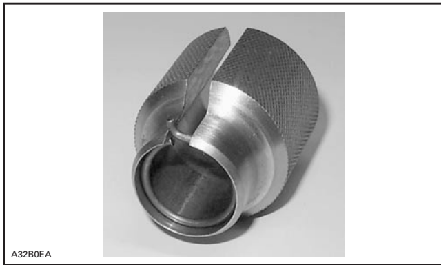
CIRCLIP READY TO BE INSTALLED ON PISTON
