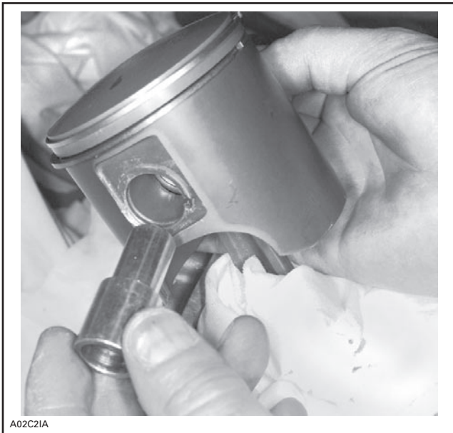
TYPICAL — SHOULDERED SLEEVE INSTALLATION
