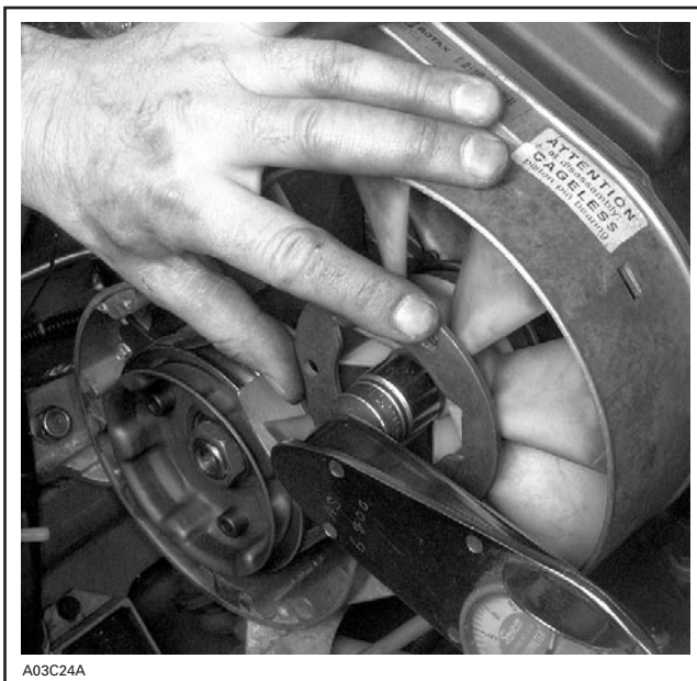
TORQUE FAN NUT USING HOLDER WRENCH
