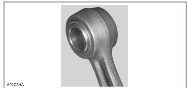
TYPICAL — CAGELESS BEARING AND SLEEVE INSTALLED
