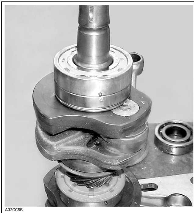
PTO SIDE BEARING FILLED WITH ISOFLEX GREASE
