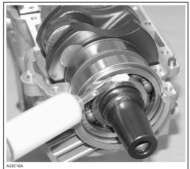
BALLS COATED WITH A SEAM OF GREASE
