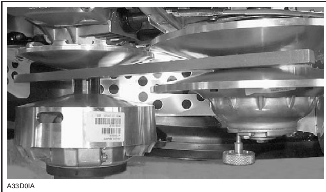
ALIGNMENT BAR IN PULLEYS
