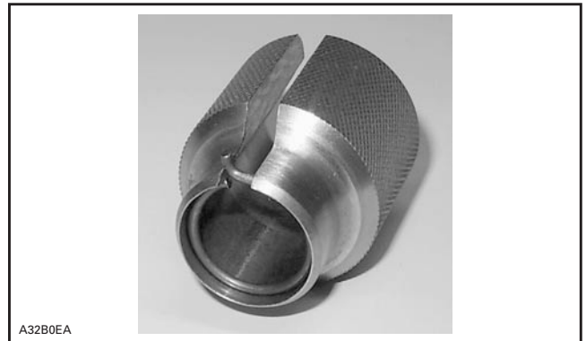
CIRCLIP READY TO BE INSTALLED ON PISTON
