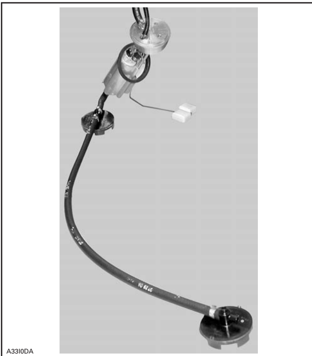
1. Fuel pickups with their strainer facing downward
