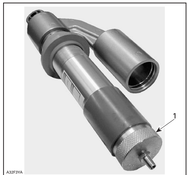
1. Floating piston remover tool (P/N 529 035 907)
