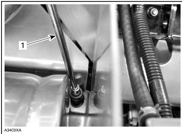
1. 14 inch-drive extension with the modified socket
