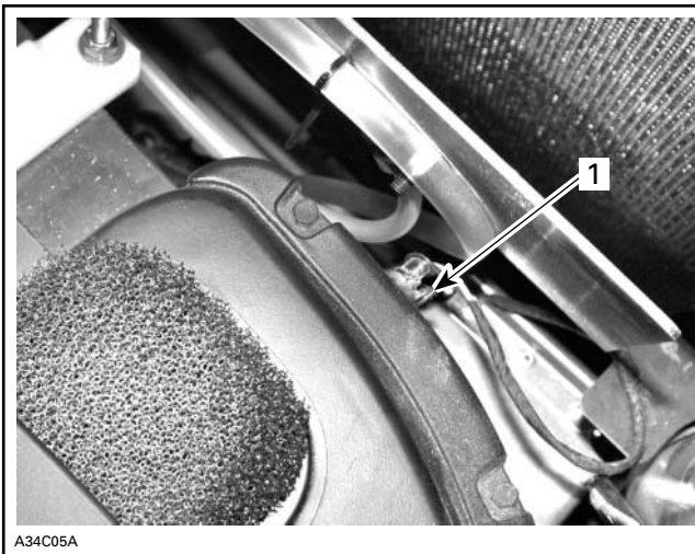
TYPICAL 1. Air temperature sensor
