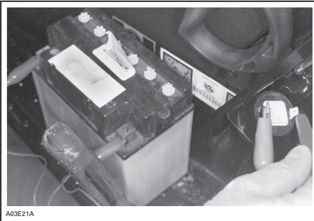
TYPICAL — 12-VOLT BATTERY PLUGGED TO BUZZER
