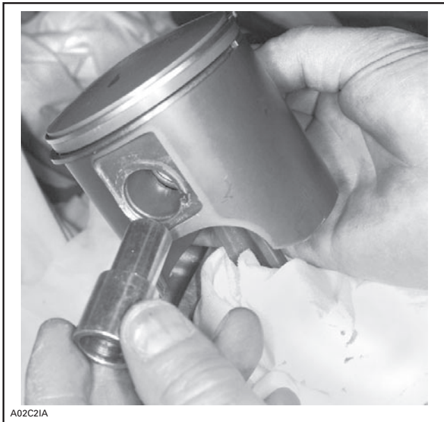
TYPICAL — SHOULDERED SLEEVE INSTALLATION
