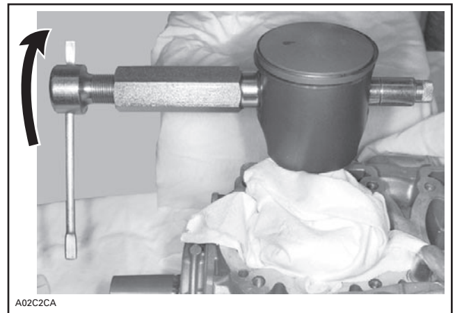
TYPICAL — PISTON PIN EXTRACTION
