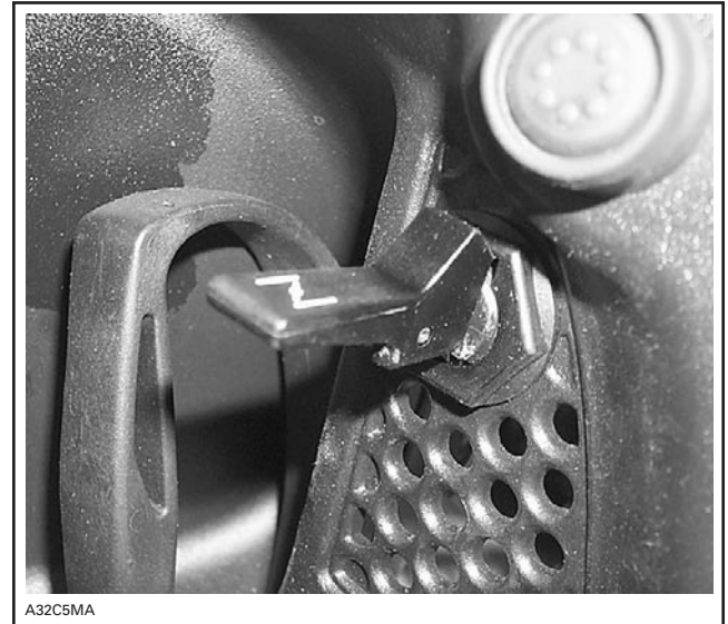
CHOKE LEVER — HALF OPEN POSITION
