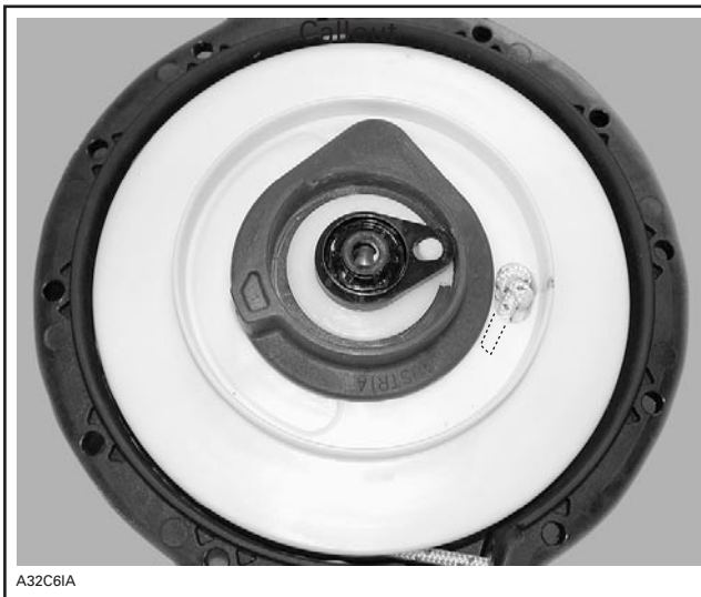
FREE PORTION INSERTED INTO SHEAVE
