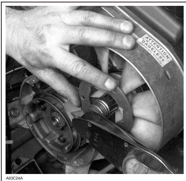
TORQUE FAN NUT USING HOLDER WRENCH
