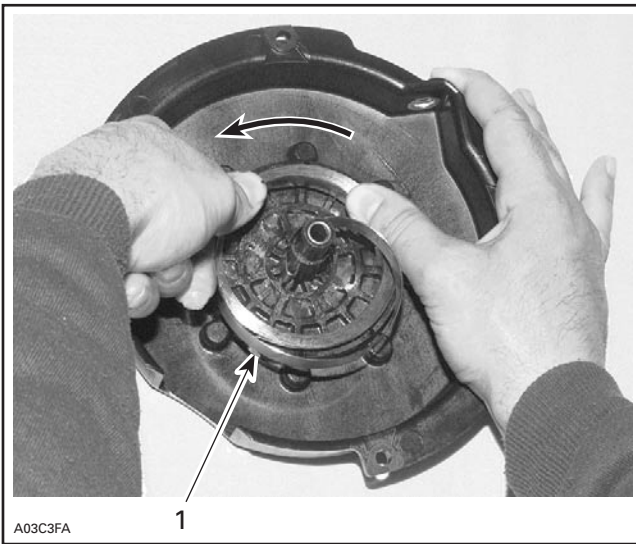
1. Outer end into guide notch
