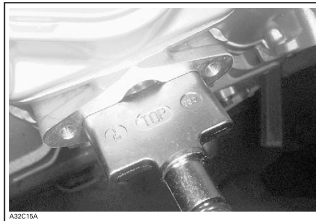
RAVE VALVE PARTIALLY REMOVED
