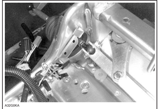
TIE ROD BALL JOINT PARALLEL TO SWIVEL BAR BEFORE TIGHTENING
