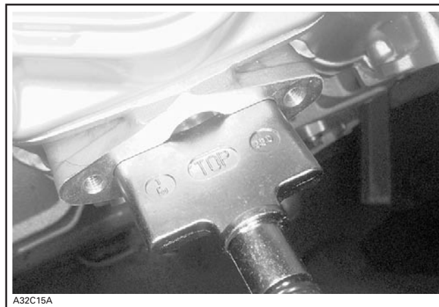
RAVE VALVE PARTIALLY INSERTED
