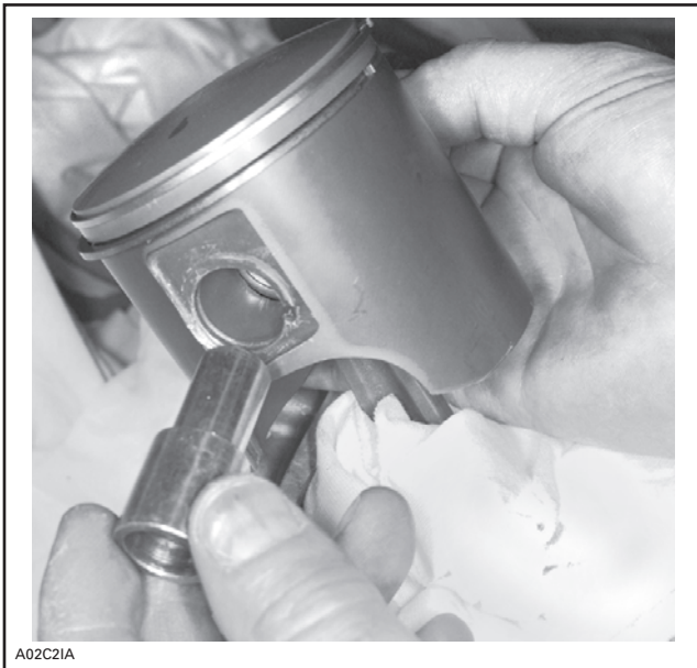
TYPICAL — SHOULDERED SLEEVE INSTALLATION
