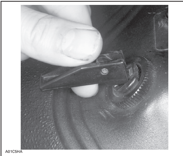
CHOKE LEVER — FULLY OPEN POSITION
