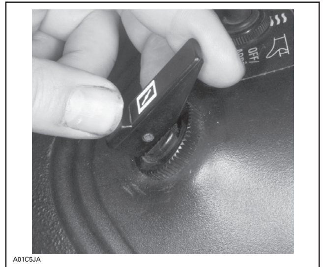
CHOKE LEVER — CLOSED POSITION
