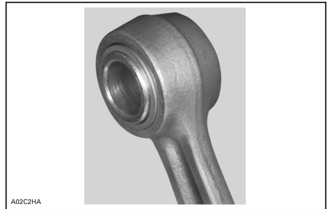
TYPICAL — CAGELESS BEARING AND SLEEVE INSTALLED
