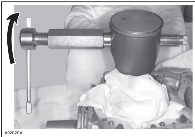
TYPICAL — PISTON PIN EXTRACTION
