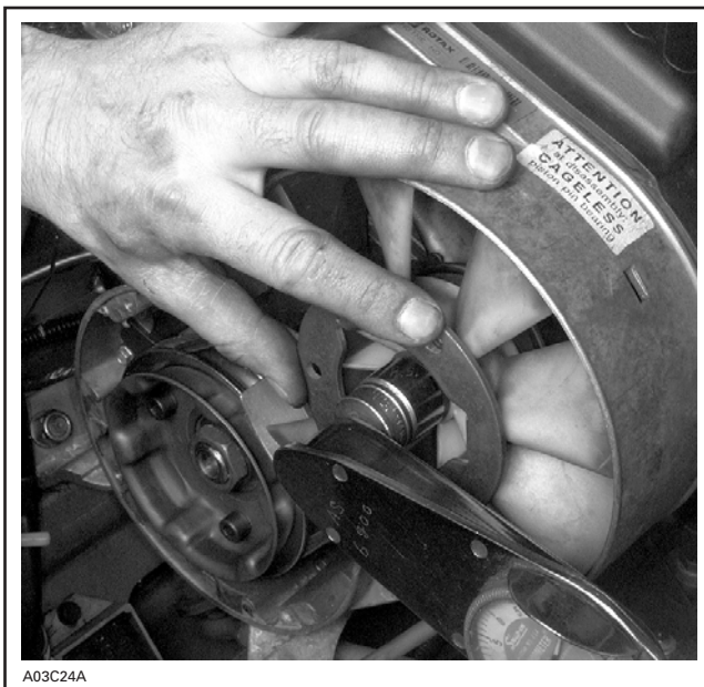
TORQUE FAN NUT USING HOLDER WRENCH
