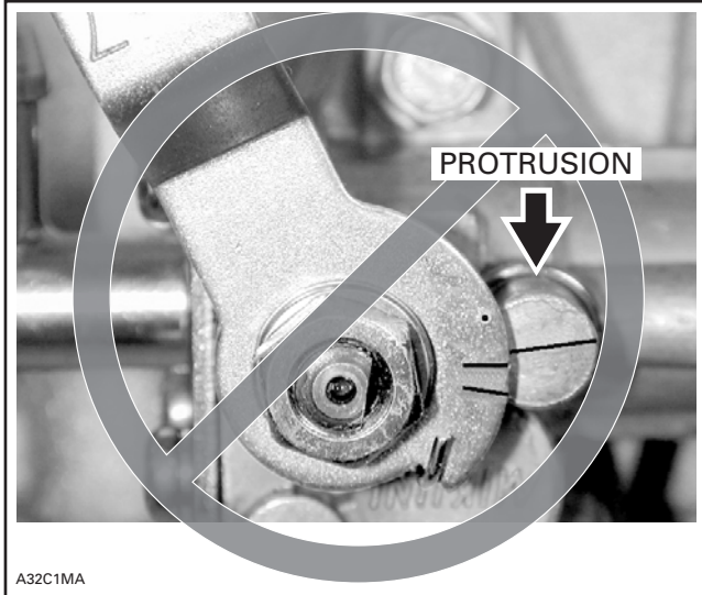
VIEW TOO HIGH — ADJUSTMENT SEEMS TO BE TOO RICH WHEN TOP OF BODY'S PROTRUSION CAN BE SEEN
