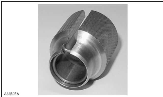
CIRCLIP READY TO BE INSTALLED ON PISTON
