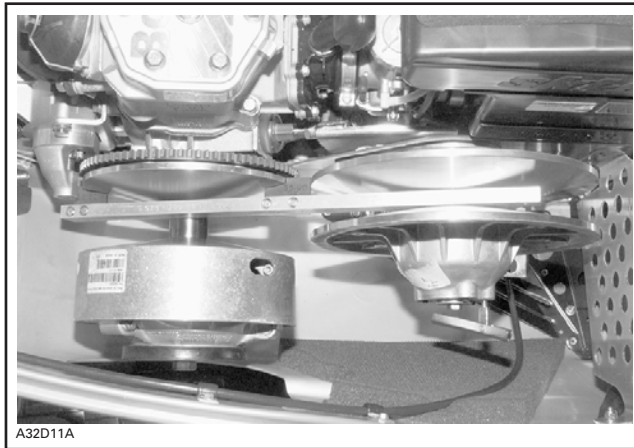
ALIGNMENT BAR IN PULLEYS
