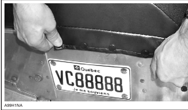
STRETCH SNAP FLAP AND MARK HOLE PLACES
