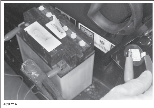
TYPICAL — 12-VOLT BATTERY PLUGGED TO BUZZER
