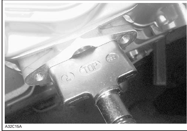
RAVE VALVE PARTIALLY REMOVED
