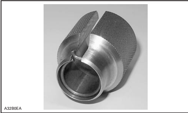
CIRCLIP READY TO BE INSTALLED ON PISTON
