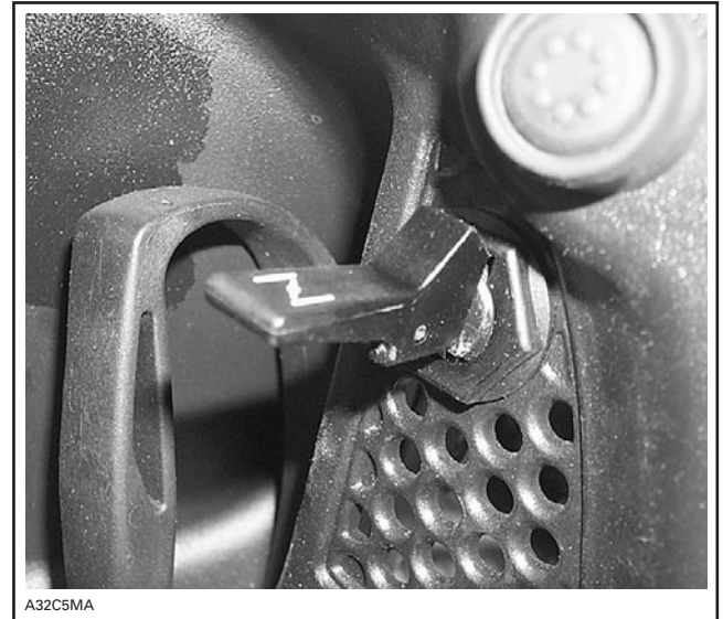
CHOKE LEVER — HALF OPEN POSITION
