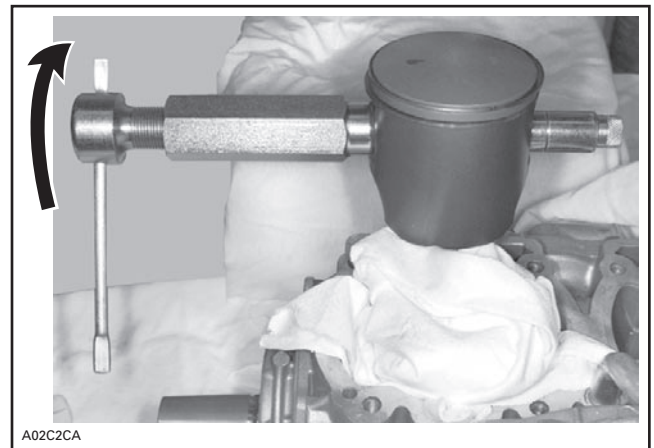
TYPICAL — PISTON PIN EXTRACTION
