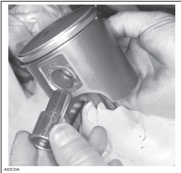
TYPICAL — SHOULDERED SLEEVE INSTALLATION
