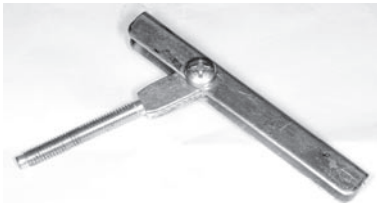
Driven pulley opening tool (P/N 529 035 501)
