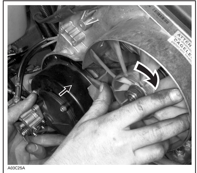
TURN FAN TO SLIDE OIL PUMP SHAFT IN PLACE
