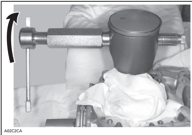
TYPICAL — PISTON PIN EXTRACTION
