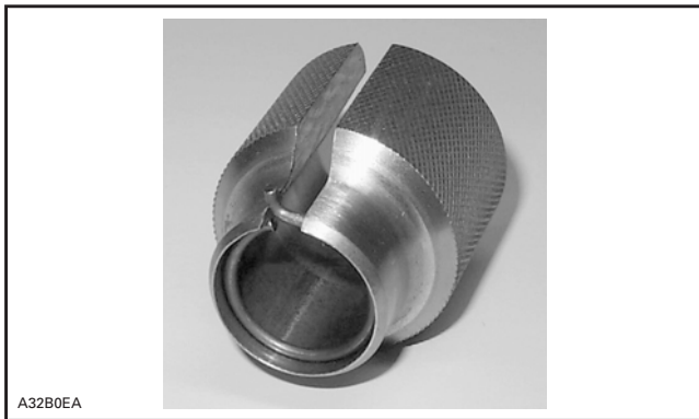
CIRCLIP READY TO BE INSTALLED ON PISTON
