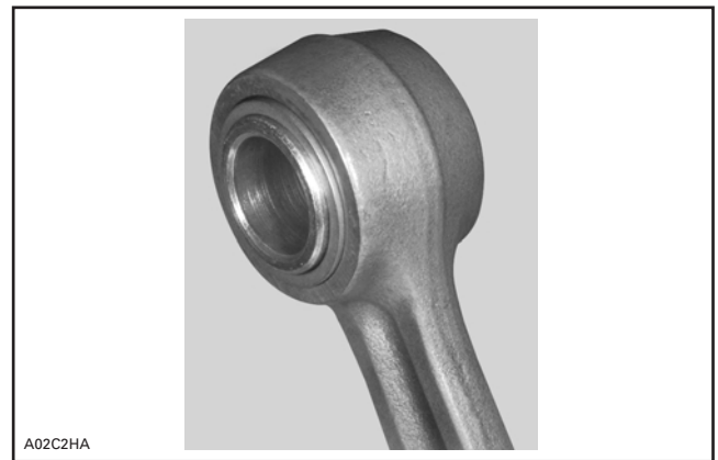
TYPICAL — CAGELESS BEARING AND SLEEVE INSTALLED
