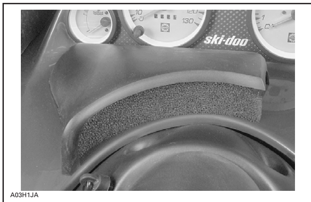
TYPICAL — FILTER INSTALLED
