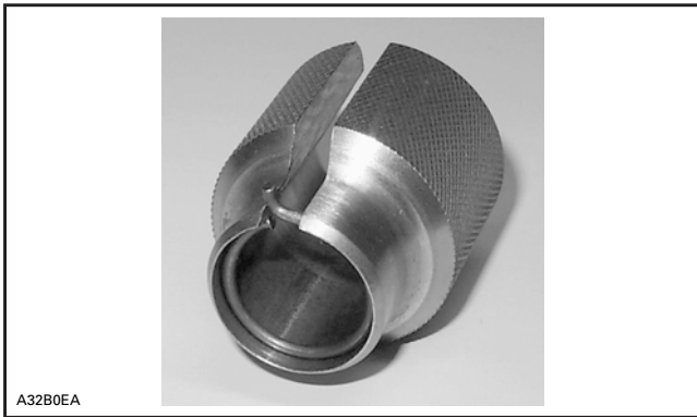
A32B0EA CIRCLIP READY TO BE INSTALLED ON PISTON
