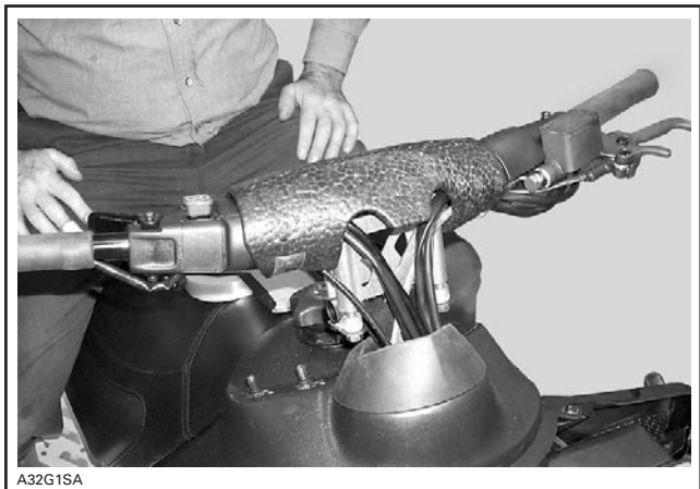
STEERING FOAM TEMPORARILY INSTALLED WITH FILAMENT TAPE
