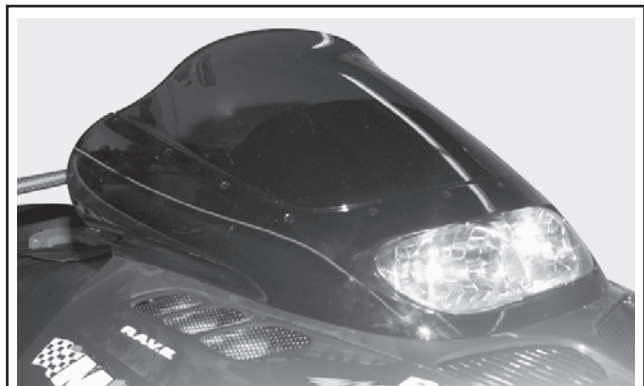
A06H3GA TYPICAL — WINDSHIELD INSTALLED ON DASHBOARD
