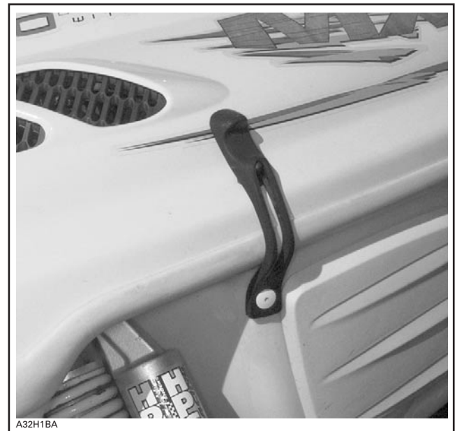
1. Drill and rivet stud 2. Drill and rivet latch
