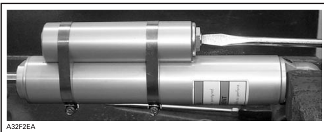
DISCHARGING GAS PRESSURE
