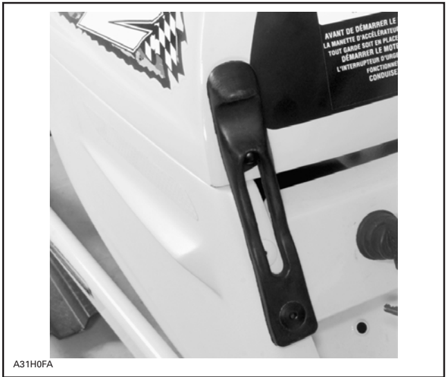
LEFT SIDE SHOWN — HOOD LATCH IN FASTENING POSITION
