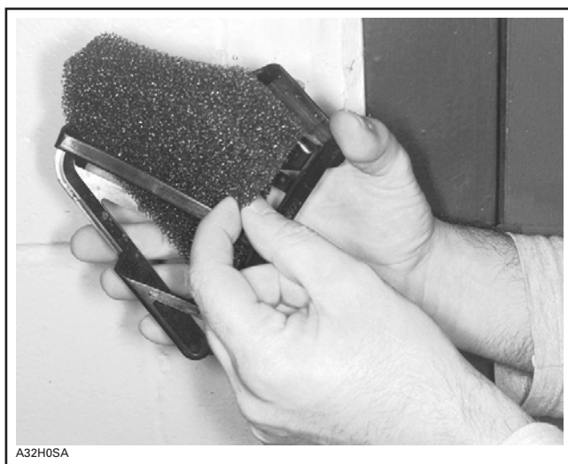
REMOVAL OF FILTER FROM ITS GRILL
