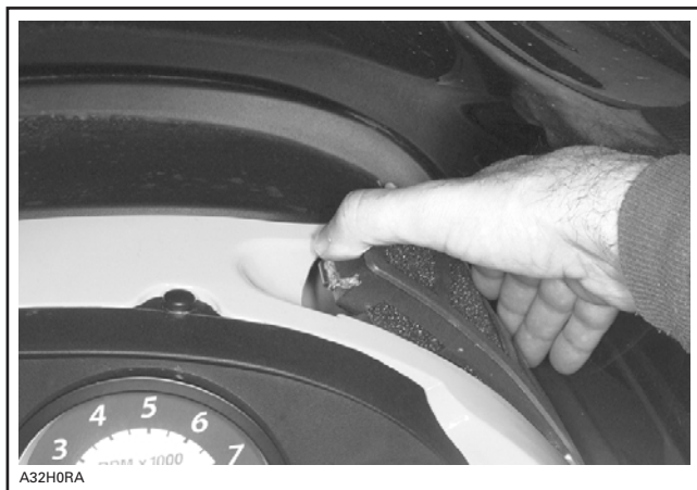
REMOVAL OF RIGHT SIDE PRIMARY FILTER GRILL
