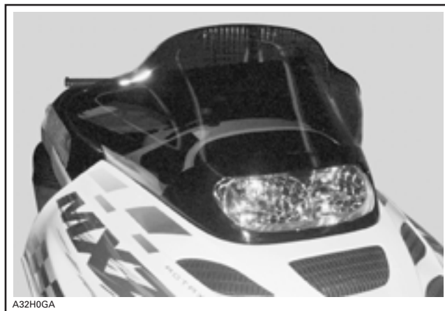
TYPICAL — WINDSHIELD INSTALLED
