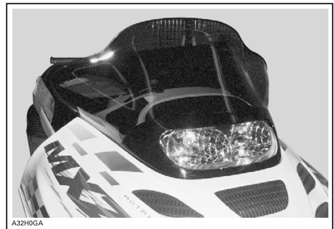
TYPICAL — WINDSHIELD INSTALLED
