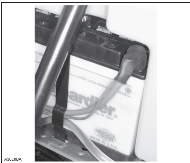
RED POSITIVE (+) BATTERY CABLE AND WIRE POSITIONING
