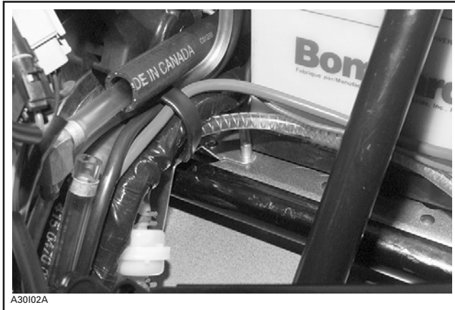
VENT TUBE PROPERLY CONNECTED
