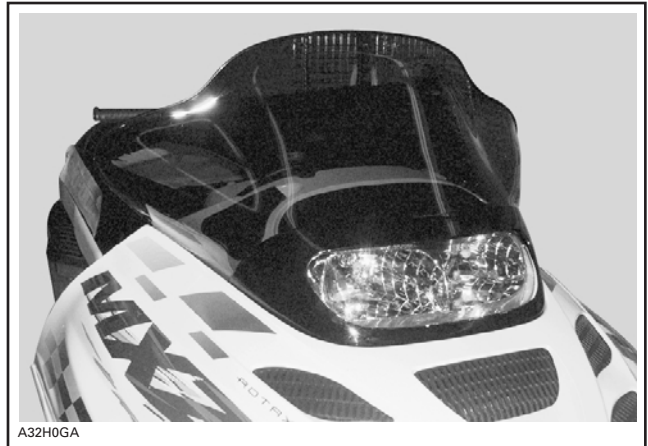
TYPICAL — WINDSHIELD INSTALLED
