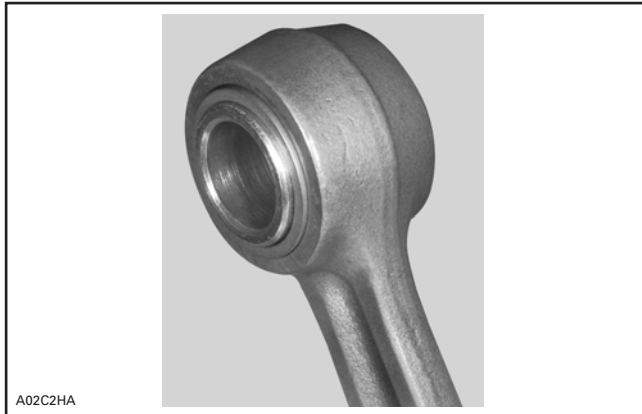
TYPICAL — CAGELESS BEARING AND SLEEVE INSTALLED
