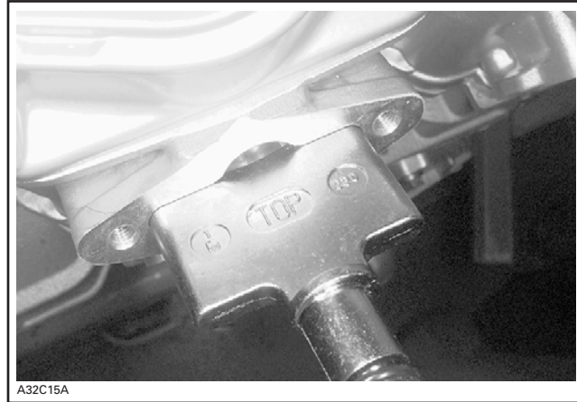
RAVE VALVE PARTIALLY REMOVED
