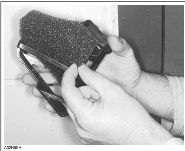
REMOVAL OF FILTER FROM ITS GRILL
