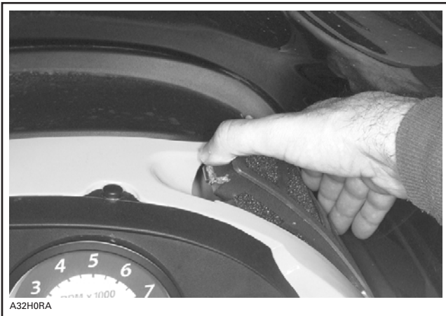
REMOVAL OF RIGHT SIDE PRIMARY FILTER GRILL
