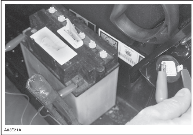
12-VOLT BATTERY PLUGGED TO BUZZER
