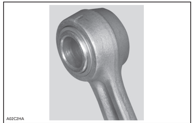
TYPICAL — CAGELESS BEARING AND SLEEVE INSTALLED
