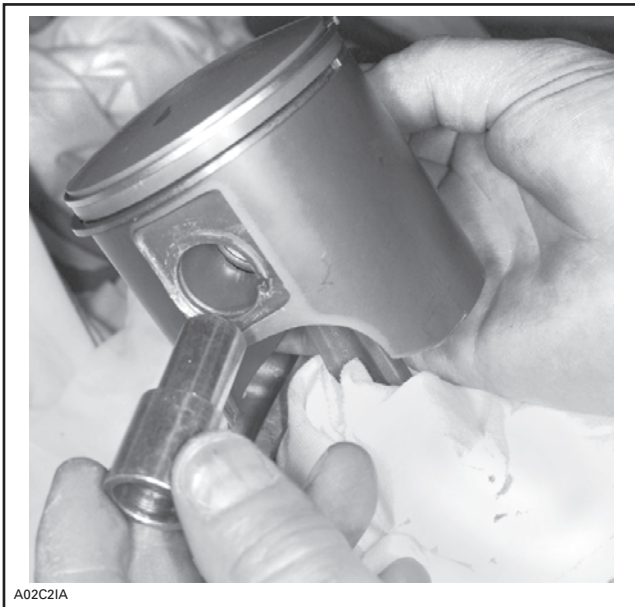
TYPICAL — SHOULDERED SLEEVE INSTALLATION
