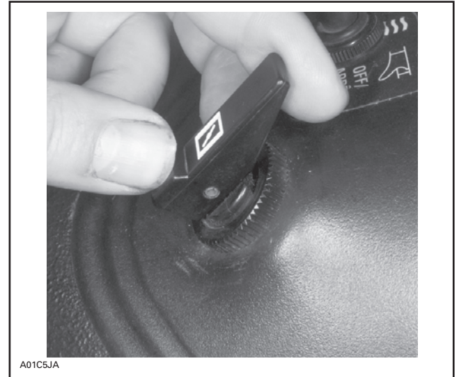
CHOKE LEVER — CLOSED POSITION
