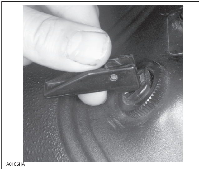
CHOKE LEVER — FULLY OPEN POSITION
