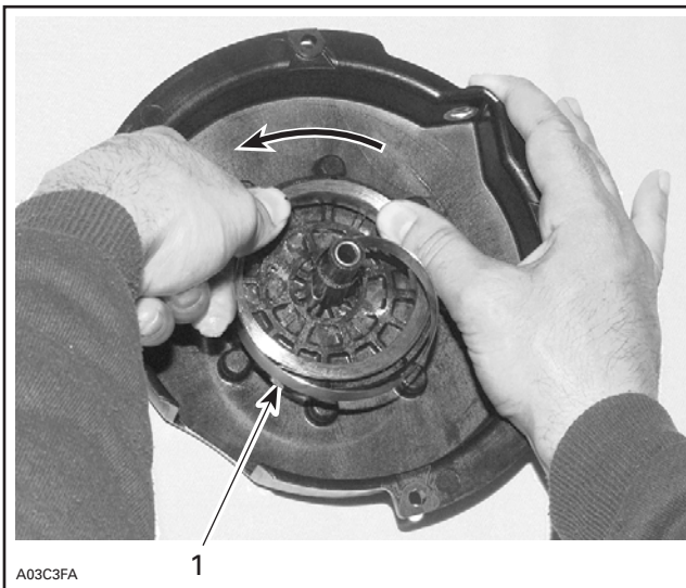
1. Outer end into guide notch
