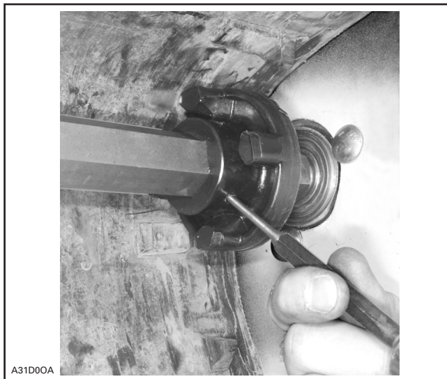
REMOVE SPRING PIN
