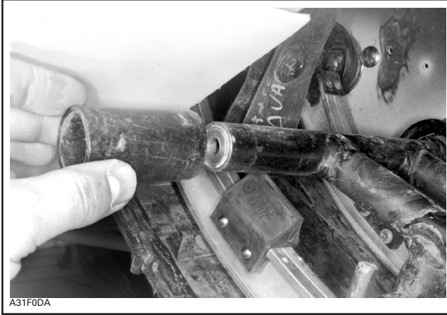
REMOVE AND CLEAN BUSHING
