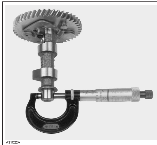
MEASURE CAMSHAFT OUTSIDE DIAMETER
