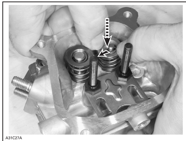
TYPICAL — PUSH DOWN AND SLIDE RETAINER TO THE SIDE
