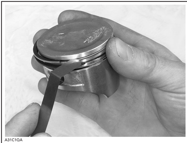
RING/PISTON GROOVE CLEARANCE
