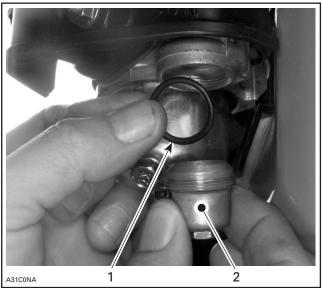
REMOVE STRAINER CUP 1. O-ring 2. Strainer cup
