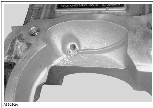
METAL CHIPS AFTER DRILLING (TO BE REMOVED)
