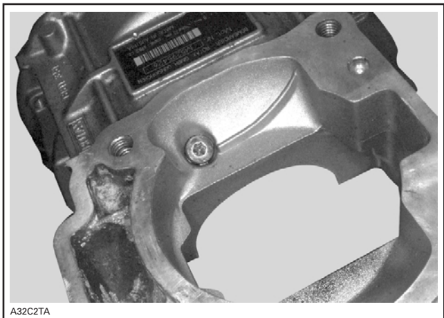
HOLE BLOCKED WITH SCREW
