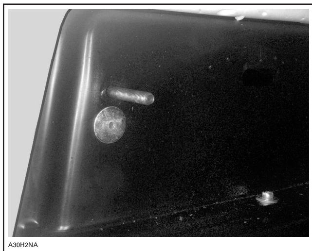
SHOWS "PLATE WITH SCREW" ALREADY RIVETED
