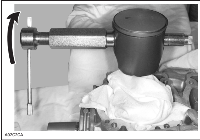
TYPICAL — PISTON PIN EXTRACTION
