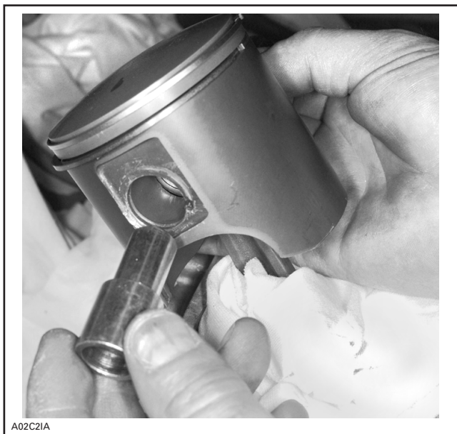
TYPICAL — SHOULDERS SLEEVE INSTALLATION
