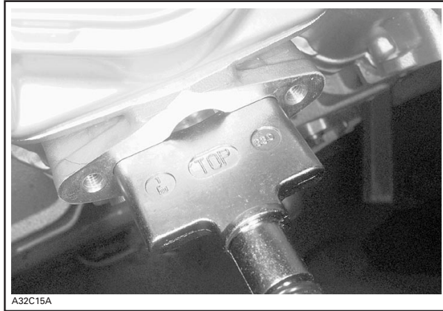
RAVE VALVE PARTIALLY REMOVED
