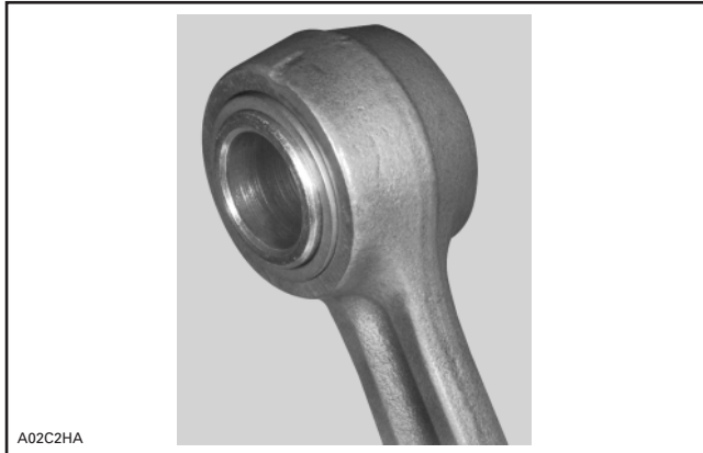
TYPICAL — CAGELESS BEARING AND SLEEVE INSTALLED
