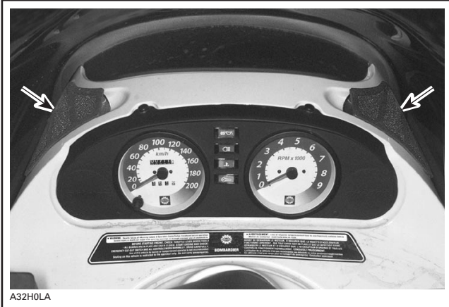
PRIMARY FILTER LOCATION
