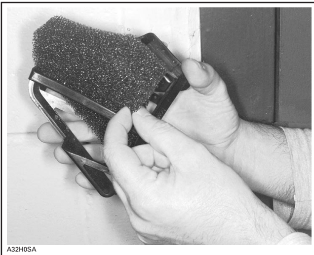
REMOVAL OF FILTER FROM ITS GRILL
