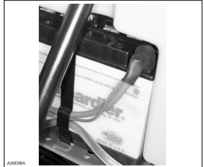
RED POSITIVE (+) BATTERY CABLE AND WIRE POSITIONING
