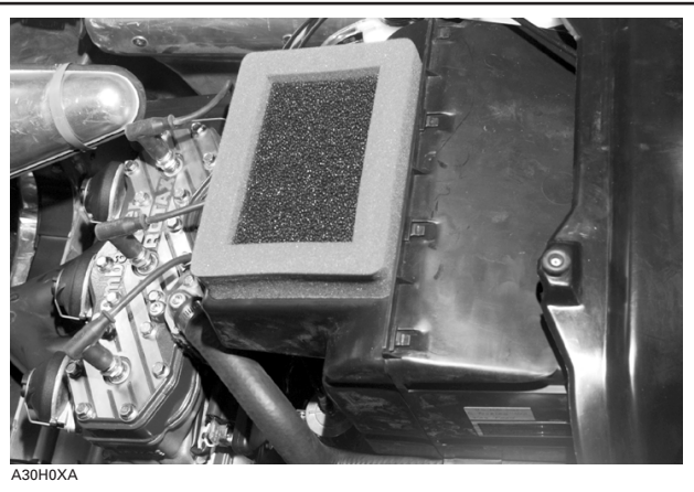
AIR FILTER INSTALLED
