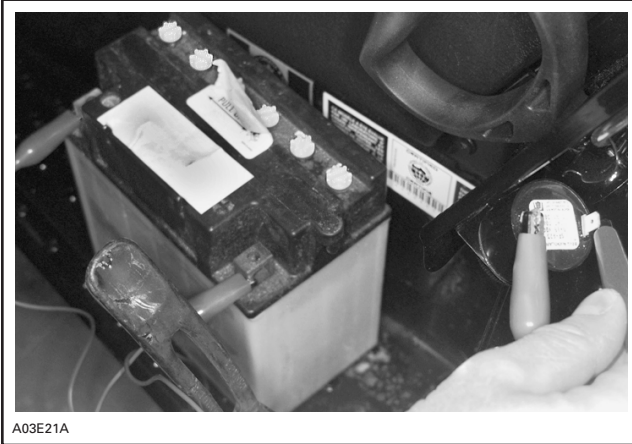
12-VOLT BATTERY PLUGGED TO BUZZER
