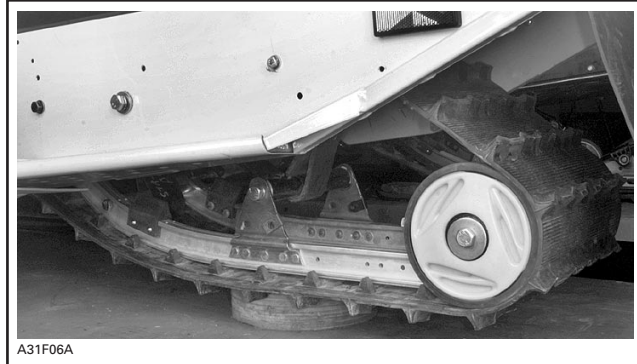
POSITION A SMALL BLOCK BELOW TRACK
