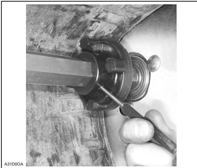
REMOVE SPRING PIN
