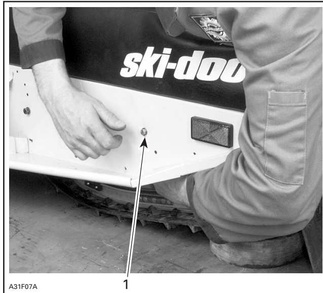
1. Unscrew upper idler wheel axle
