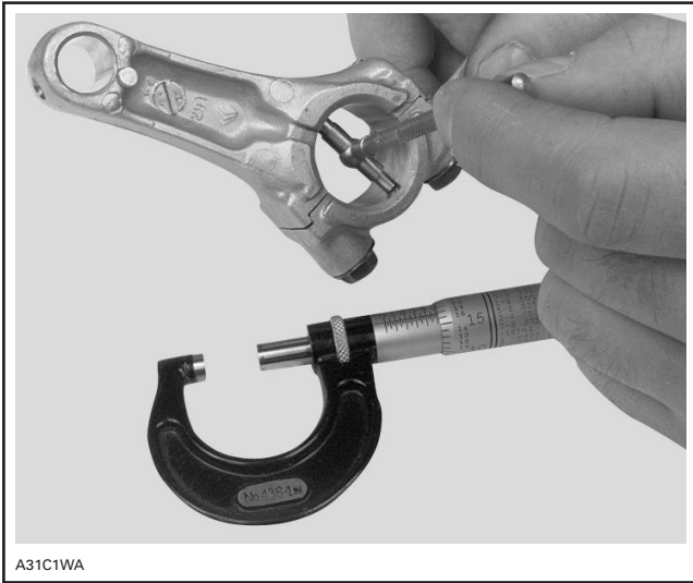
MEASURE CONNECTING ROD BIG END
