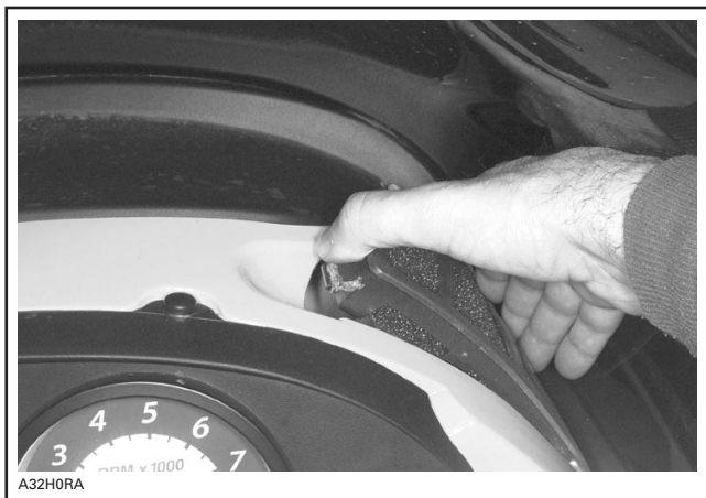
REMOVAL OF RIGHT SIDE PRIMARY FILTER GRILL
