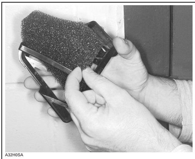
REMOVAL OF FILTER FROM ITS GRILL
