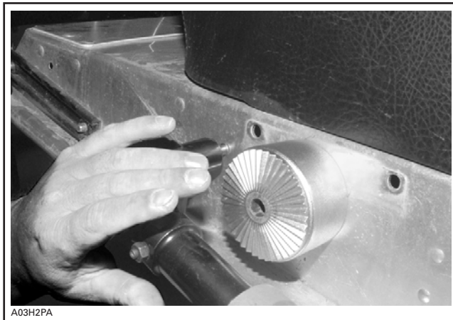
RIVET BRACKET FROM OUTSIDE TUNNEL
