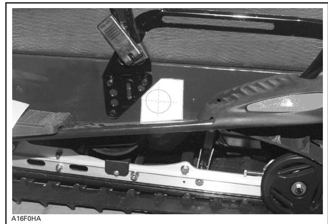
Using center punch, mark the hole position. Drill a 18 mm (0.709 in) hole.
