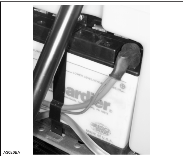
RED POSITIVE (+) BATTERY CABLE AND WIRE POSITIONING
