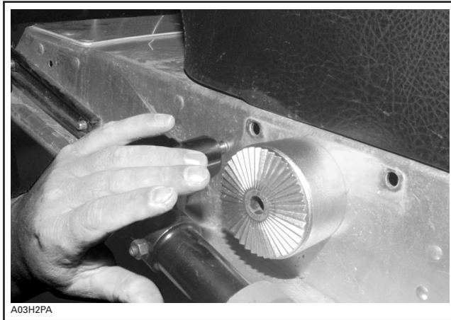
Rivet bracket from outside tunnel
