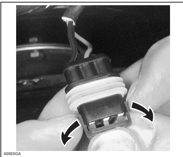
LIFT BOTH TABS THEN REMOVE CONNECTOR CAP
