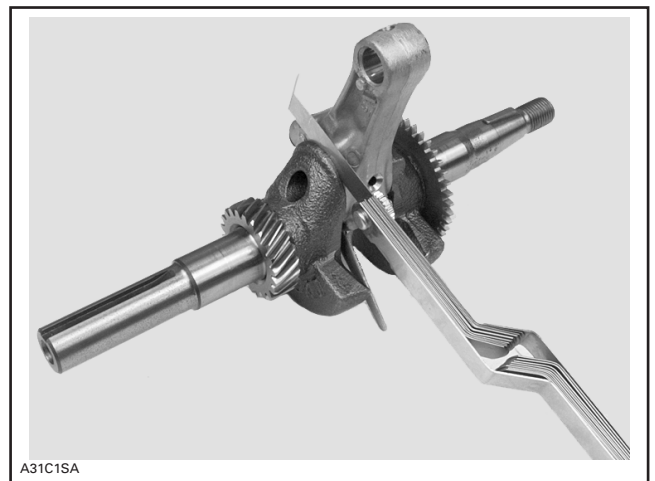
MEASURE SIDE CLEARANCE
