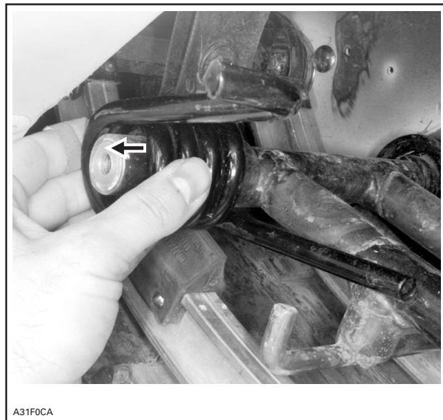
REMOVE TORSION SPRING
