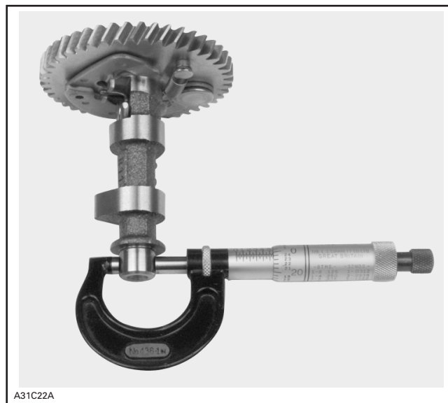
MEASURE CAMSHAFT OUTSIDE DIAMETER
