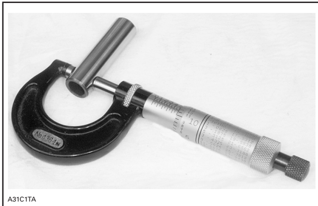
MEASURE PISTON PIN
