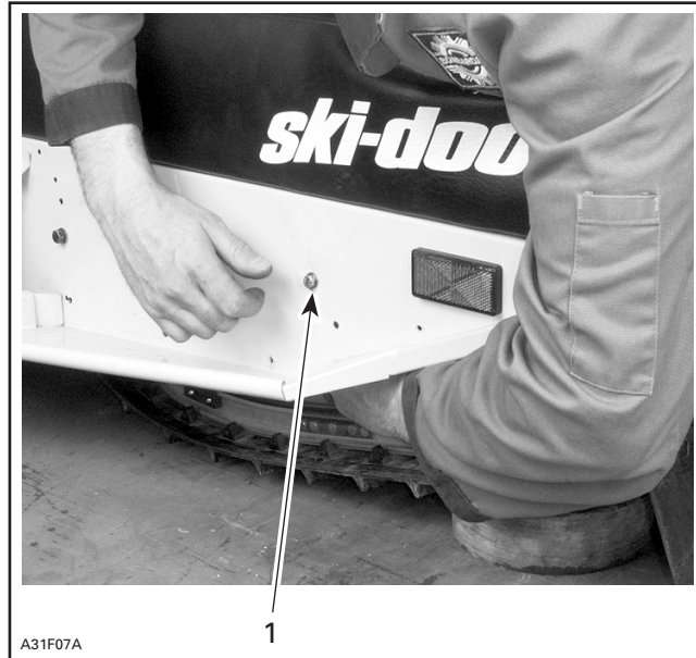
1. Unscrew upper idler wheel axle
