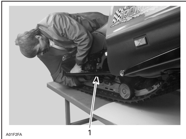
1. Remove hook on the rear portion of the suspension
