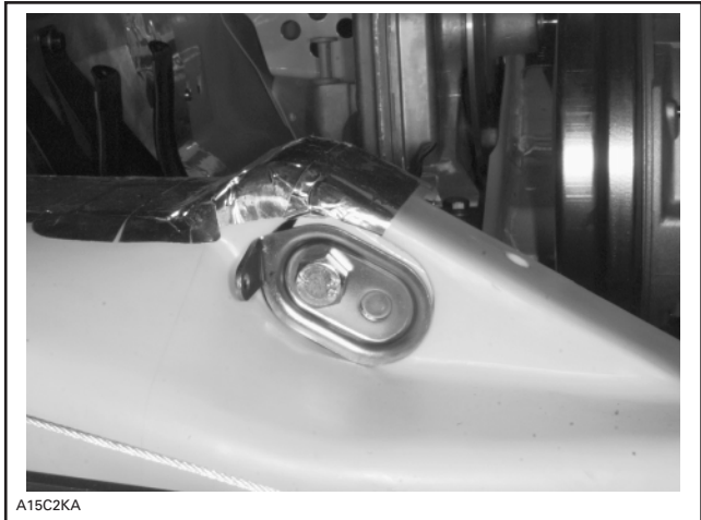
EXHAUST SUPPORT PROPERLY INSTALLED
