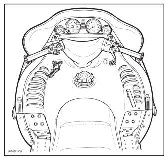
**Steering** - The steering handlebar assembly controls the direction of travel of the snowmobile. As the handlebar is rotated to right or left, the skis are turned in the direction of intended travel. Proper shifting of your body weight helps in turning. Occasionally check your steering system to be sure its movement is unrestricted.
