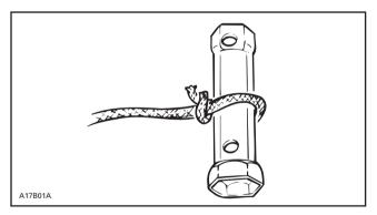
Wind the rope tightly around drive pulley. When pulled, pulley must rotate counterclockwise.
