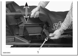
1. Lift adjustment lock (both sides)
