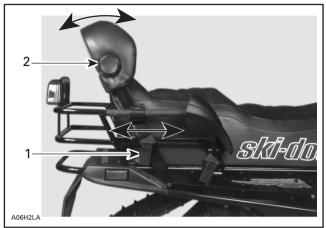
1. Lift adjustment lock (both sides)
