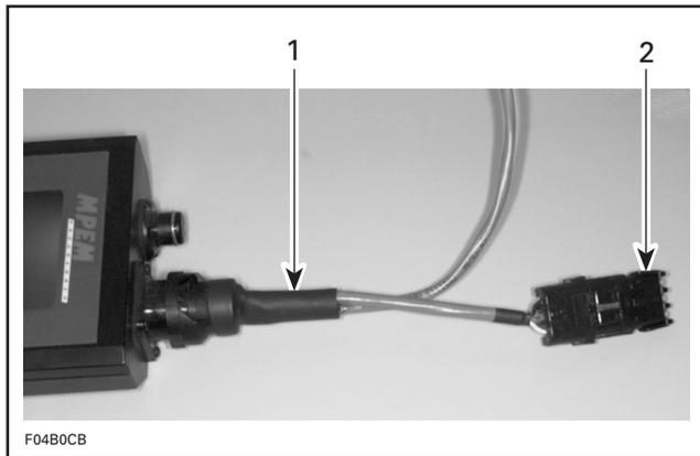
1. MPEM cable plugged to MPEM programmer
