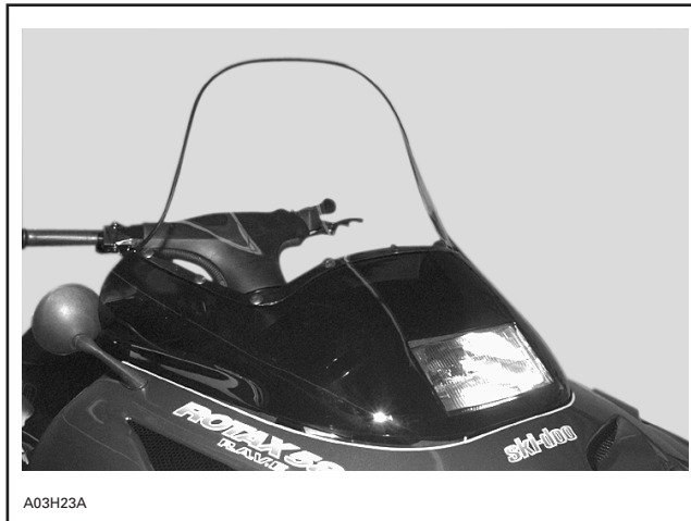
WINDSHIELD INSTALLED ON DASHBOARD
