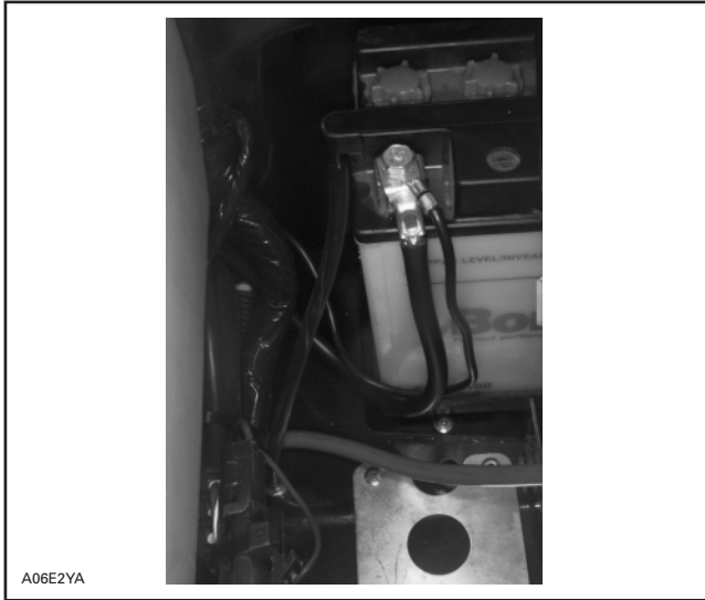
BLACK NEGATIVE (-) BATTERY CABLES POSITIONING
